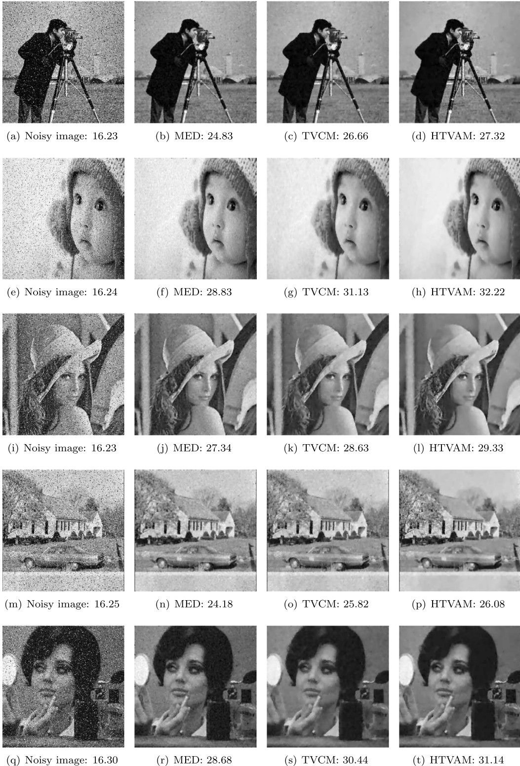
Fig. 4. Denoising results of three methods at \varepsilon = 0.04 (each value in parentheses represents the corresponding PSNR (dB) value of the restored image). From left to right: the noisy images, MED, TVCM, and HTVAM.
