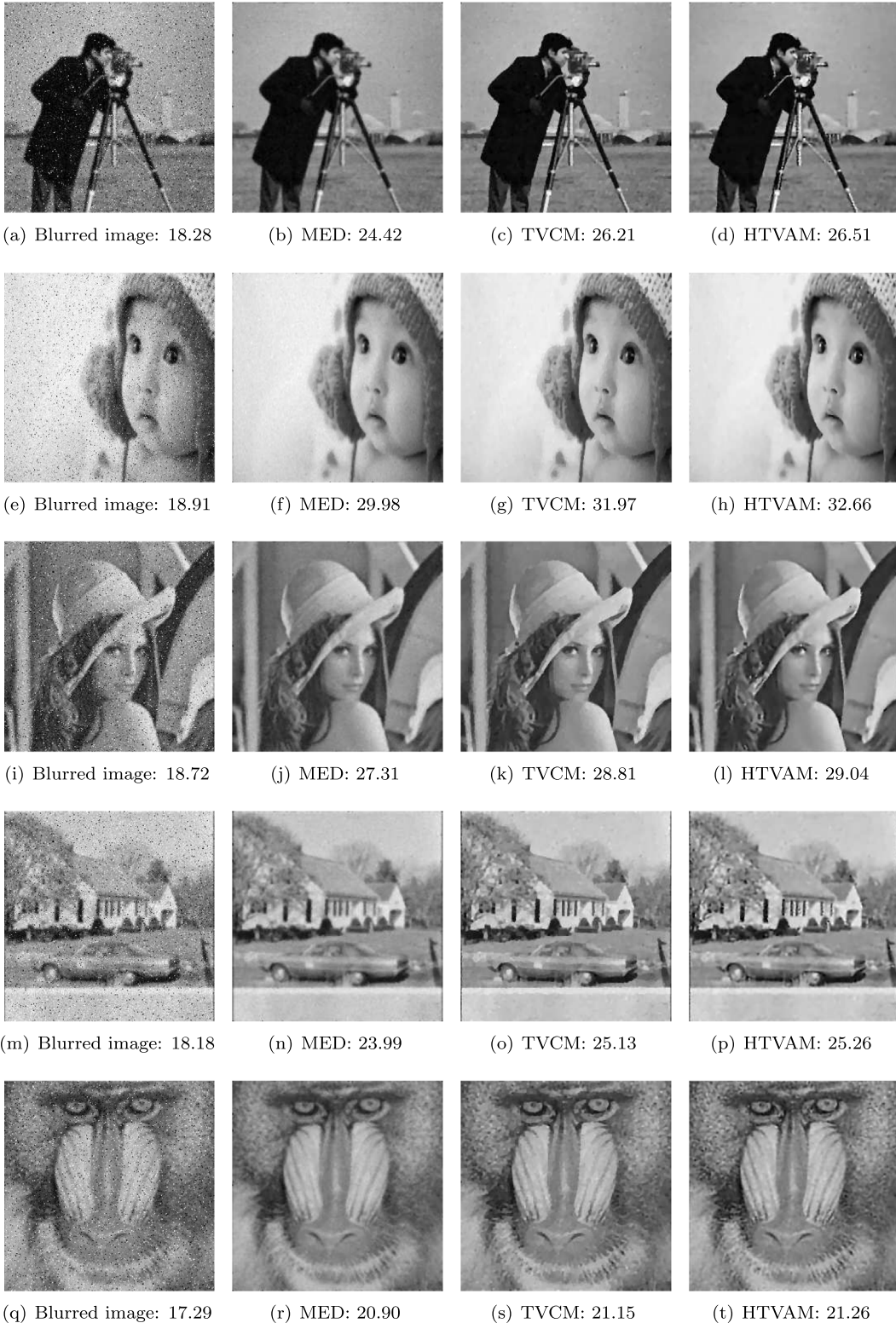
Fig. 6. Restoration results of different methods for blurred images with Cauchy noise at \varepsilon = 0.02 (each value in parentheses represents the corresponding PSNR (dB) value of the restored image). From left to right: the blurred images with Cauchy noise, MED, TVCM, and HTVAM.
